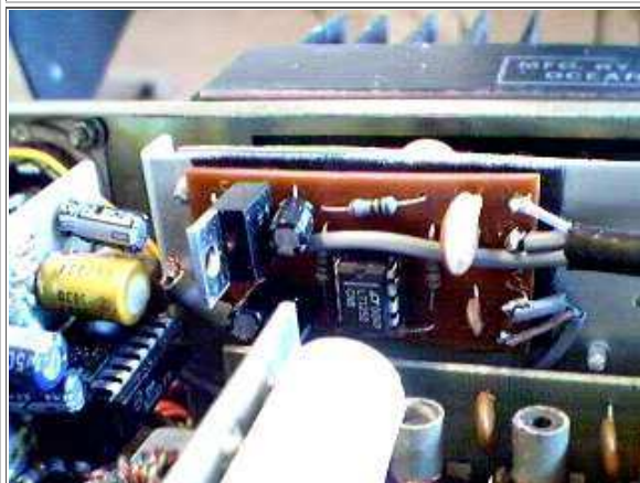
Atlas210 preamp board installation
