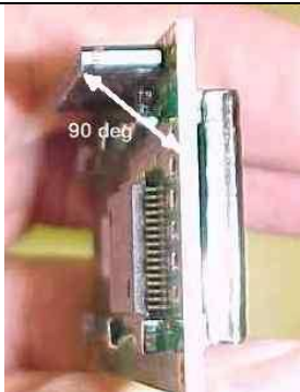
solder the female 14 pin connector in pins 1-14 of the display module
